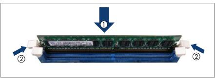
Figure 36: Installing a memory module
